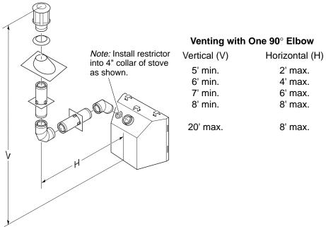
Figure 26 - Vertical Rigid Venting Configuration Using One 90° Elbow Continued
